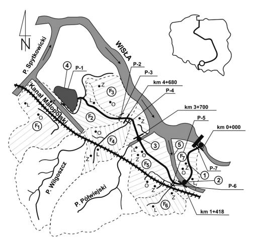
**Fig. 1.** Łączany draining system subdivided into sub-cachments. Soil sampling sites are marked: O - arable land, L - forests - Z - grassland, T - urbanized areas
